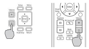
You can also press the dutten on the remote control to temporarily turn off the sound.
