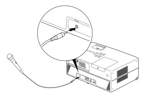
You can adjust the volume using the projector's volume controls on the control panel or remote control. If the microphone level is too low, you can adjust it by pressing the button on the remote control or through the Option menu (see page 51).
