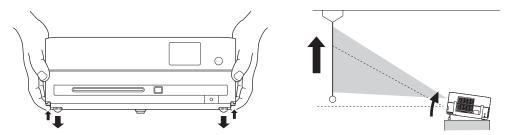
■ If the image is horizontally tilted, you can turn the feet to level it.
