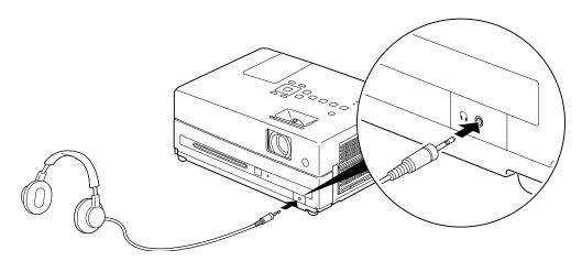
After you connect headphones, you no longer hear any sound from the built-in speakers. However, you can still adjust the volume to the headphones using the projector's volume controls on the control panel or remote control.
