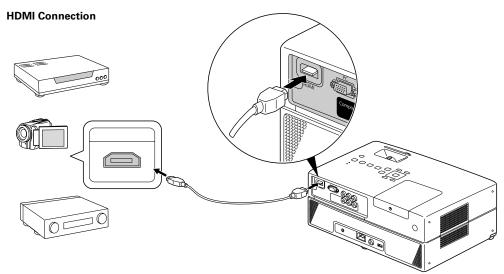
For connecting an HD cable or satellite TV receiver, HD DVR, or HD camcorder.
