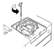
5. Grasp the lamp handle as shown and pull the lamp straight out.
